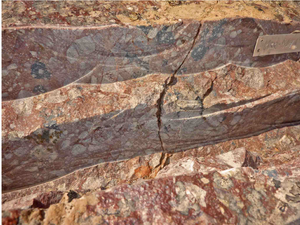
(Fig 5- Channel saw sample showing strong hydrothermal brecciation and hematite matrix. Two samples were collected here as a check on variability within vein and for possible near surface silver enrichment. Metal 2" sample tag on right for scale)
